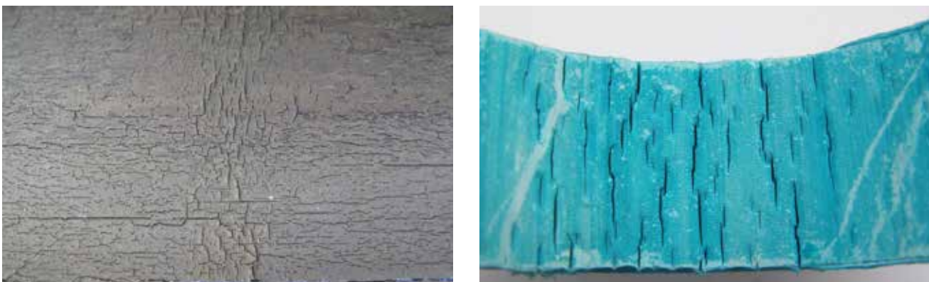
Signs of chemical aggression occurred since a thermoplastic material not suitable for the transported fluid was chosen.
