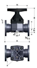
**VMOM** Diaphragm valve with flanged monolithic body, drilled EN/ISO/DIN PN10/16. Face to face according to EN 558-1
