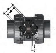
**Power Quick Easyfit**The valve can be equipped with pneumatic or electric standard actuators and gearboxfor heavy-duty operations, using the PP-GR module reproducing the drilling pattern foreseen by ISO 5211.
