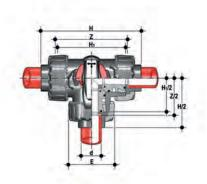
LKDIM DUAL BLOCK® 3-way ball valve with metric plain socket ends for socket welding, - L bore.
