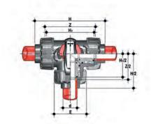
DUAL BLOCK  $^{\scriptscriptstyle \otimes}$  3-way ball valve with metric plain socket ends for socket welding, - T bore.
