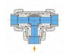
B - T-port ball valve: 90° - Diverting
