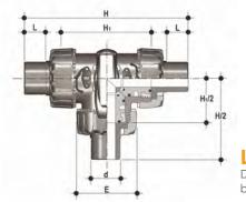
LKDDM DUAL BLOCK® 3-way ball valve with male ends for socket welding, metric series, L-port ball.
