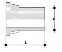
End connectors in PP-H SDR 11 PN 10, long spigot, for butt welding
