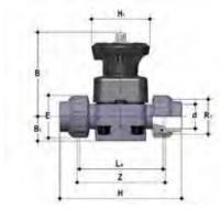
**DKUAV**DIALOCK® diaphragm valve with female union ends for solvent welding, ASTM series
