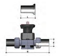
**Q/BBE-L**Long spigot PE100 end connectors for electrofusion or butt welding
