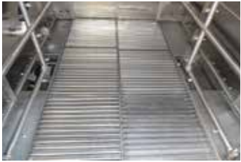
Stainless steel rack washer now completely scale free
