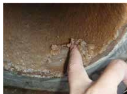
The scale in the circulation pipe can also be easily removed with a finger.
