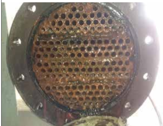
Heat exchanger before Vulcan installation
