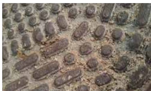
After Vulcan was installed only for 1 month, the scale is softened and falling off.
