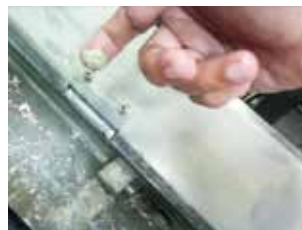
June 13 : The Machine 2 with Vulcan for 1 month, the scale has been dissolved and can be removed with a finger.
